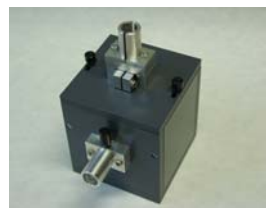
A box, with the input and exit ports, containing the integrating sphere. The sphere (about 80 mm diameter) is coated with a reflective silver layer and covered with a white vitrified paint.
