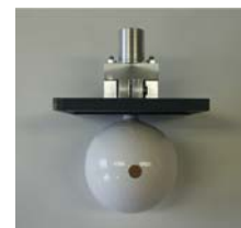
The sphere is fixed to the top cover plate of the box. The support for the optical fibre is on the top, the input window is on the front side of the sphere.
